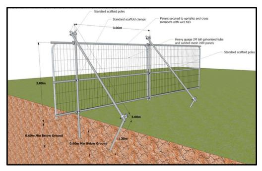
Figure 4: Default specification for tree protection barrier in accordance with BS5837:2012 figure 2
